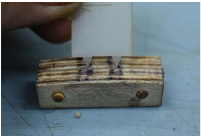
15. To glue a vortex generator. Slip the fin into the oval. Place into the jig, press down and add a clamp.
