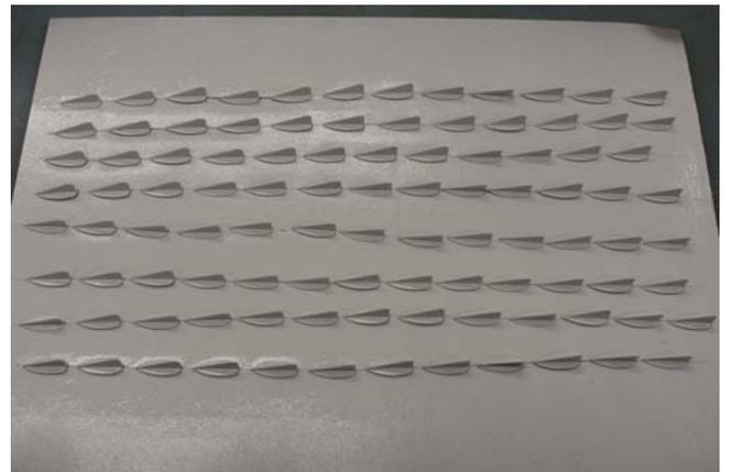
19. Cut long slices in corrugated cardboard (parallel with the corrugations) and stick them into the slices for priming and painting. **Do Not Use The Piercing Tool** for this, the tips will break off.
