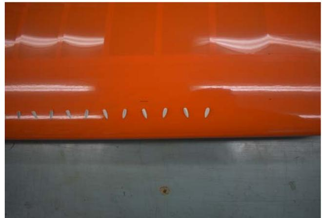
**28.** Move the template over as shown on STEP 7 on the drawing. The open end sits onto the last glued vortex generator. Repeat steps 23 through 26 for these last five vortex generators.
