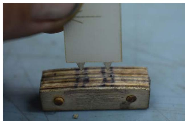
18. There are extra vortex generators supplied. Check the bottom for any excessive glue blobs and cut away.
