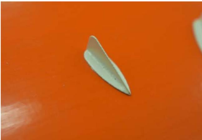
**27.** Move the template over as shown on STEP 6 on the drawing. The open end sits onto the last glued vortex generator. The template is not long enough so use another straight edge to line up the mark at the wing tip. Repeat steps 23 through 26 for this line of vortex generators.
