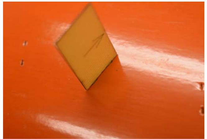
25. Dry install the vortex generators and check that they sit properly onto the wing.
