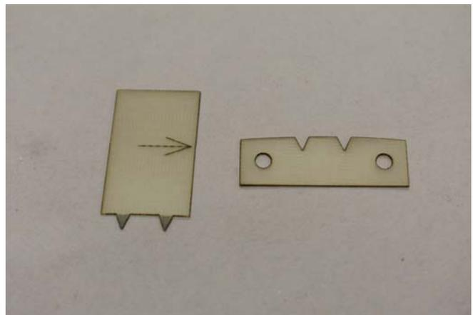
5. Use the piercing tool to push out the tiny rectangles that might be stuck in the template.
