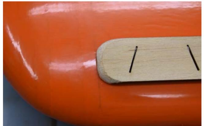
30. 1/4" balsa protectors are provided. Check fit and chamfer edges. Round over and taper at the wing tip. Label L & R with marker.
