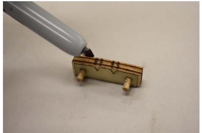
13. Assemble the other half of the gluing jig and continue the marked lines across the top.
