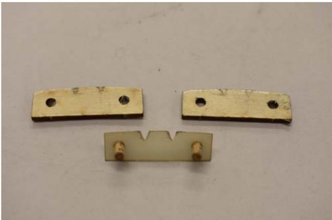
11. **Do Not Glue The Jig Together!** Slip the dowels through the G-10 piece followed by the packing tape lined lite ply part (tape is towards the G-10 part) followed by a non taped lite ply piece.
