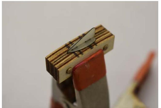
16. Using Thick or Medium CA glue with a fine applicator tip run a small bead along both sides then immediately press down on the fin so it conforms to the curvature of the jig. Hold and hit it with an accelerator.
