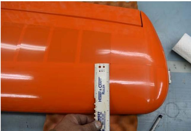
**22.** Tape the template to the wing as shown in STEP 4 on the drawing. The arrows on the template points towards the leading edge. The first picture shows the start of the template at the root of the wing.
