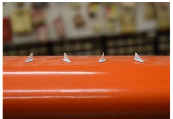
**26.** Glue in each vortex generator one at a time by adding a line or bead of CA glue between the slots and in both slots. Insert and hold vortex generator for a few moments. Continue with the next one. STEP 5 on dwg.
