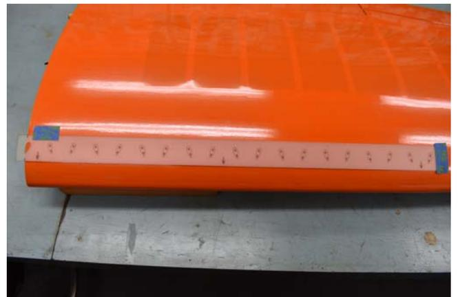
**23.** Use an X-Acto knife first to slice the covering and balsa sheeting down the center of the rectangular slots. Slice all the way through the thickness of the skin. Then use and insert the piercing tool. Do this for all the locations on the template.
