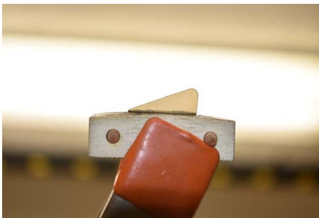
17. Somewhere between 10 to 20 units made, you may need to take apart the jig to clean it from build up of glue. Periodically use the piercing tool to check the V notch depth. Re tape the two lite ply pieces if needed.
