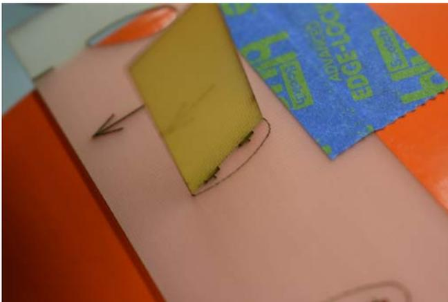
24. Remove the template and re-pierce the slots bottoming out the tool onto the sheeting.
